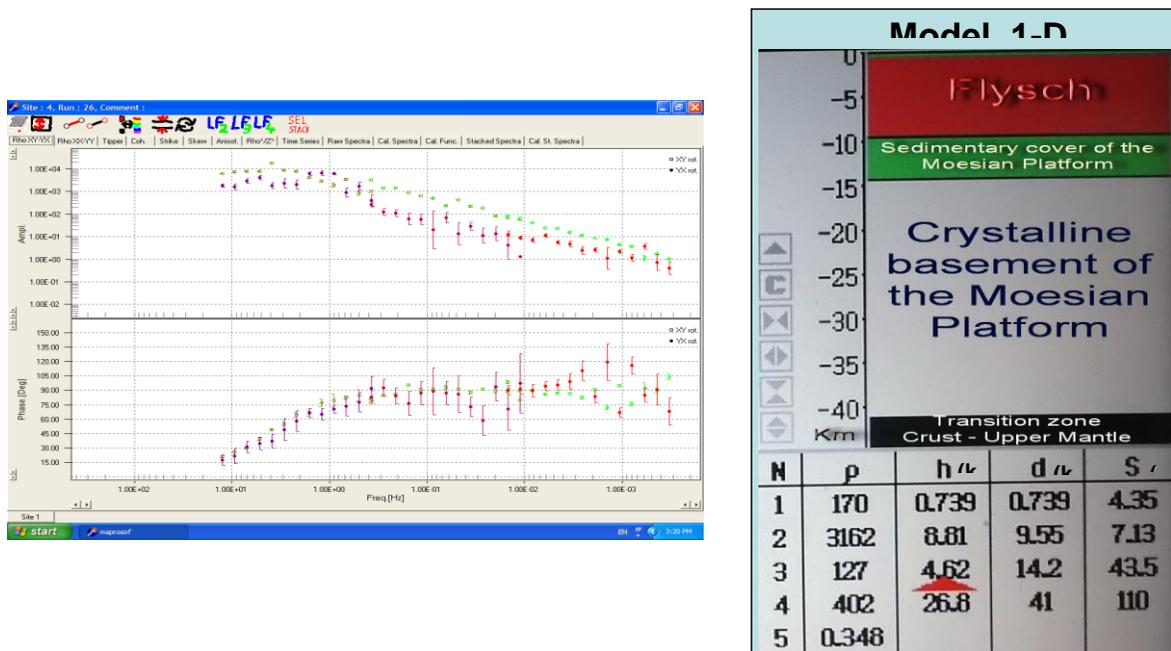
Figure 1.2.1. Left: resistivity (up) and phase (down) distributions against frequency for the magnetotelluric station Lopătari. Right: 1-D model of electrical properties
